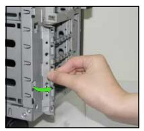
7. Secure the bracket with two screws in the holes indicated.
